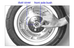
Turn bearing inner race to inspect sliding. Replace it with a new one in case of no sliding or damage or loosening of outer race.
