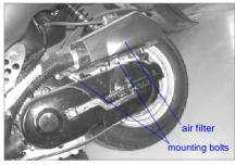
Remove mounting bolt connecting rear shock absorber and motorcycle frame, bolt connecting rear shock absorber
