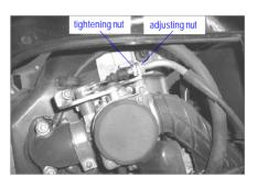
Fine adjustment is effected on the side of the thrott Effected adjustment is by removing the dust loosening the tightening nut and turning the adjusting r
