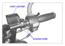
Remove brake light switch and brake lever. Remove retaining ring from main cylinder.
