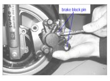
Remove two pieces of brake block pins by mear hexagon wrench.
