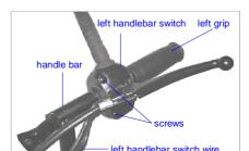
Remove 2 screws of left handlebar switch. Remove left handlebar switch. Remove left grip from handlebar.
