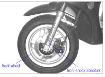
Remove 4 pieces of bolts on the upper part of from absorber.
