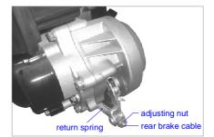
Mount brake swing arm pin and rear brake cable.
