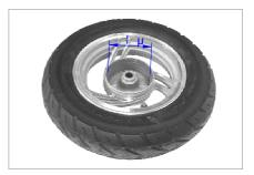
Limit of use: Ø111mm, effect replacement if the limit is exceeded.
