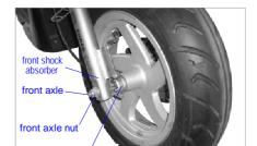
Remove front axle nut, brake calipers, front absorbers connecting bolt and remove brake calipers, front shock absorber, transmission gear box, front axle bush and the small bush, remove front axle.
