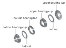
Inspect for completeness of bearing balls and if there is, effect replacement with new ones.
